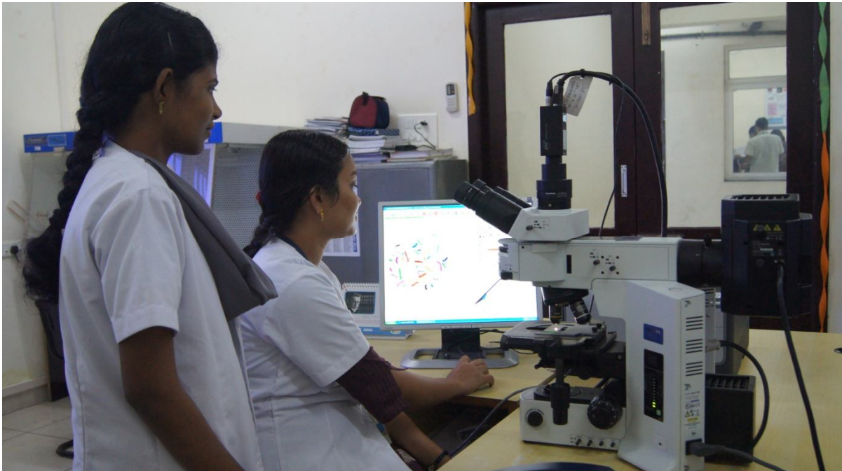
Olympus Fluorescence microscope attached with cytovision software (BX 51 model) for research and teaching
