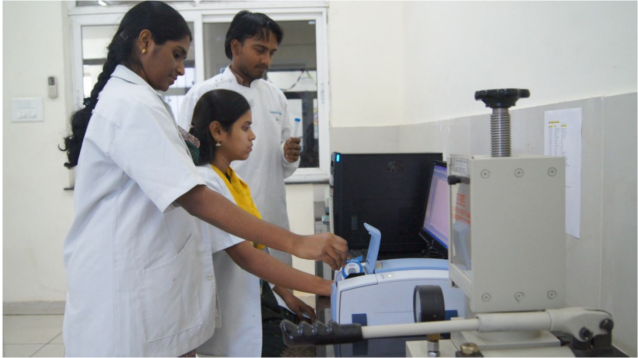
A bio nanocomposite material for medical implant is being analysed using Bruker alpha FT-IR spectrometer
