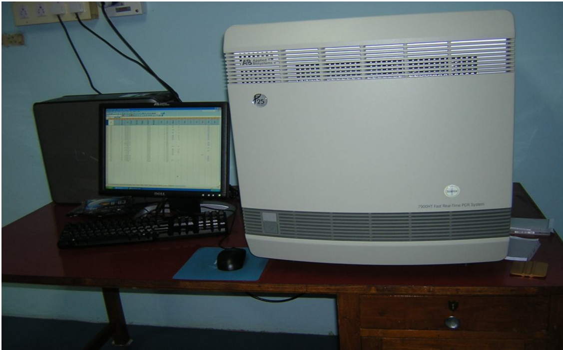
ABI 9700 HT fast real time PCR 384 well module for SNP detection, DNA quantification and melting curve analysis
