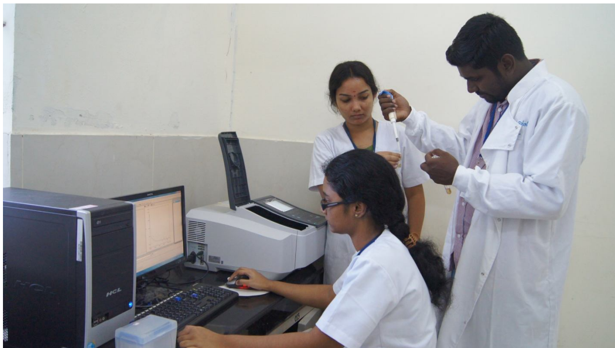
Scholars & student investigating a nano drug delivery system using Shimadzu UV-1800: UV-VIS double beam spectrophotometer
